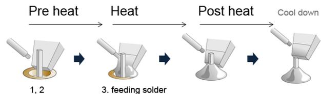
Fig.1 Iron soldering heating process
