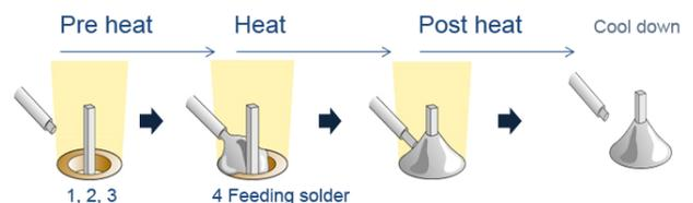
Fig. 2 Laser Soldering Heating Process
