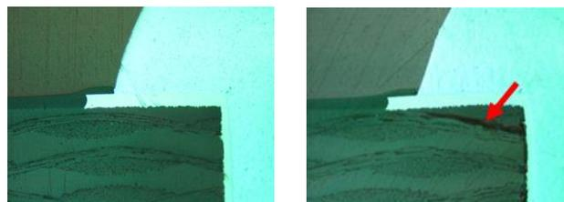
Fig 4 Comparison of effects of soldering temperature inside the substrate
