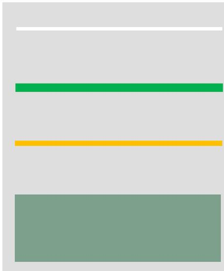
Silkscreen layer, the white oil, thickness 10~20  $\mu\text{m}$ .
