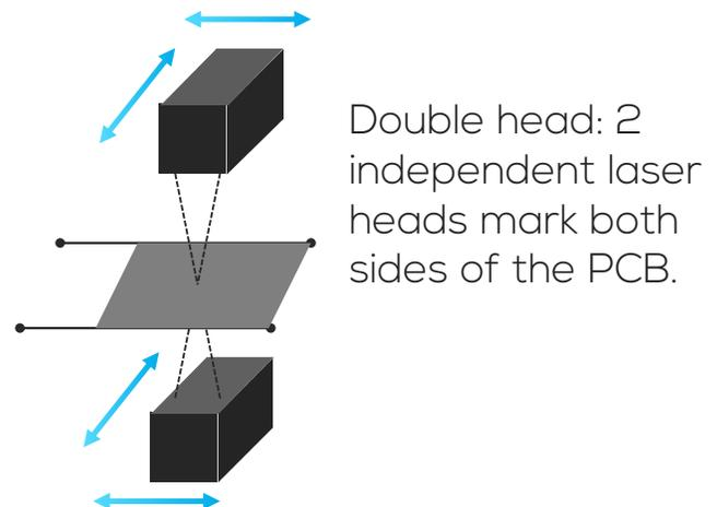
Double head: 2 independent laser heads mark both sides of the PCB.
