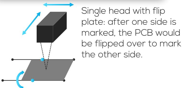
Single head with flip plate: after one side is marked, the PCB would be flipped over to mark the other side.
