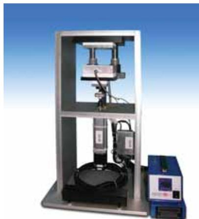
**F**ancort was approached by a well known government agency with a requirement for a very accurate, low force, assembly press that incorporated heater plates for compressing and heating semiconductor materials. The press was for R&D, and had to incorporate extreme versatility to handle the broad range of materials they were working with.
