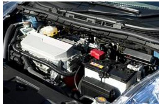
[Actuators] Due to the use of motors as actuators, there has been an increase in motors and motor drivers. Additionally, a higher number of ECU (engine control units) and DC-DC converters are added in hybrid cars.
