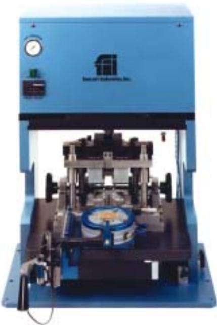
This pneumatic press enables operators to adjust all the key dimensions for lead forming, including tip-to-tip length, foot length, offset height, and bend radii.
