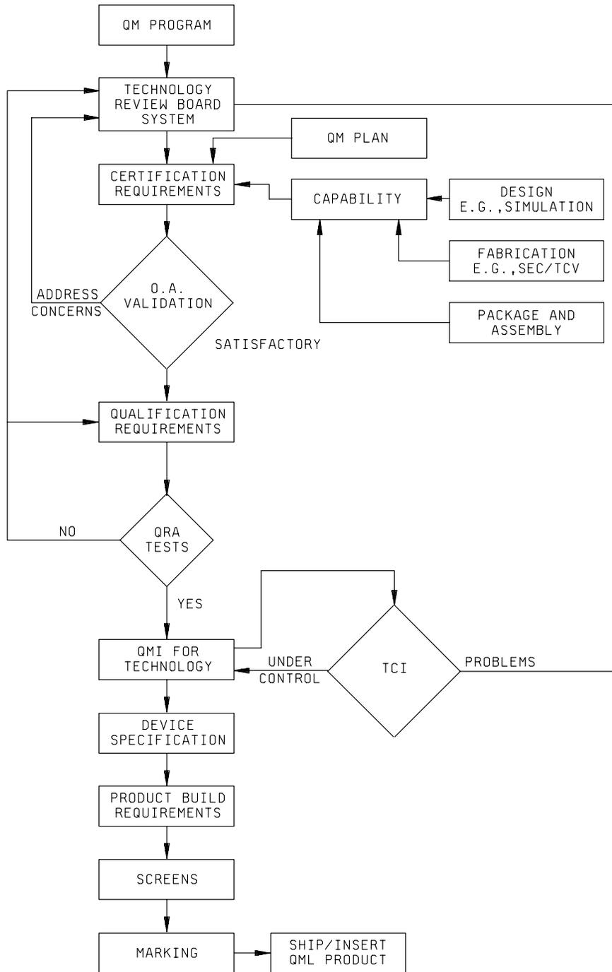
FIGURE G-1. Generic qualification flow diagram.
