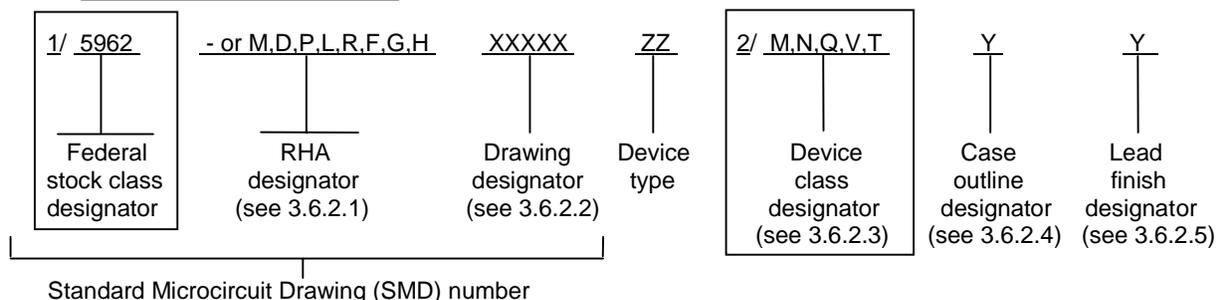
For packages where marking of the entire SMD PIN number and all other required topside marking are not possible due to space limitations, the manufacturer has the option of leaving the "5962-" off the marking. The allowance for optional marking will be indicated in the individual SMD. For RHA product using this option, the RHA designator shall still be marked.
