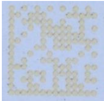
Not through mark: Marking has poor contrast
