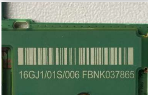
Barcode on Green Solder Mask (Green Laser)
