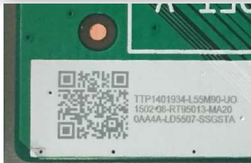
2D Barcode on White Solder Mask (UV Laser)
