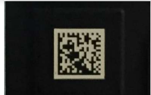
2D Barcode on Black Solder Mask
