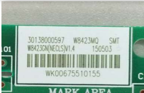
Barcode on White Solder Mask
