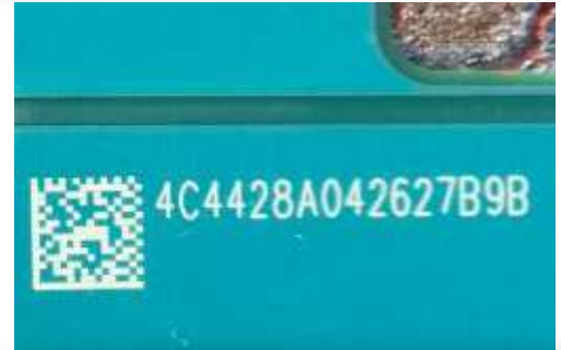
2D Barcode on Blue Solder Mask
