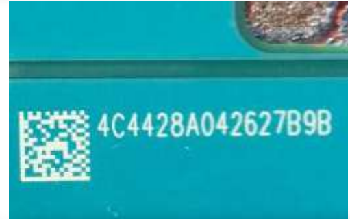
2D Barcode on Blue Solder Mask
