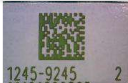
2D Barcode on White Solder Mask
