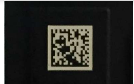
2D Barcode on Black Solder Mask
