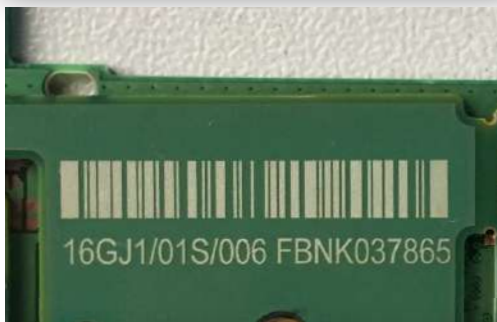
Barcode on Green Solder Mask (Green Laser)
