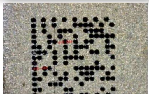
2D Barcode on Gilded Parts (Size 0.7 mm x 0.7 mm)
