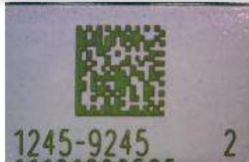
2D Barcode on White Solder Mask
