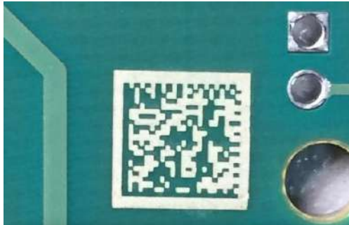
2D Barcode on Green Solder Mask
