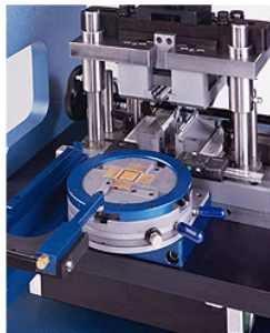
Part is lifted from the centering stage with the vacuum arm by the operator.
