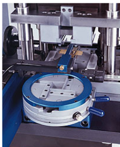
Perfectly center part is placed into the tool using the vacuum arm.
