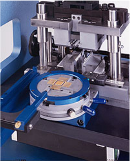
Part is lifted from the centering stage with the vacuum arm by the operator.
