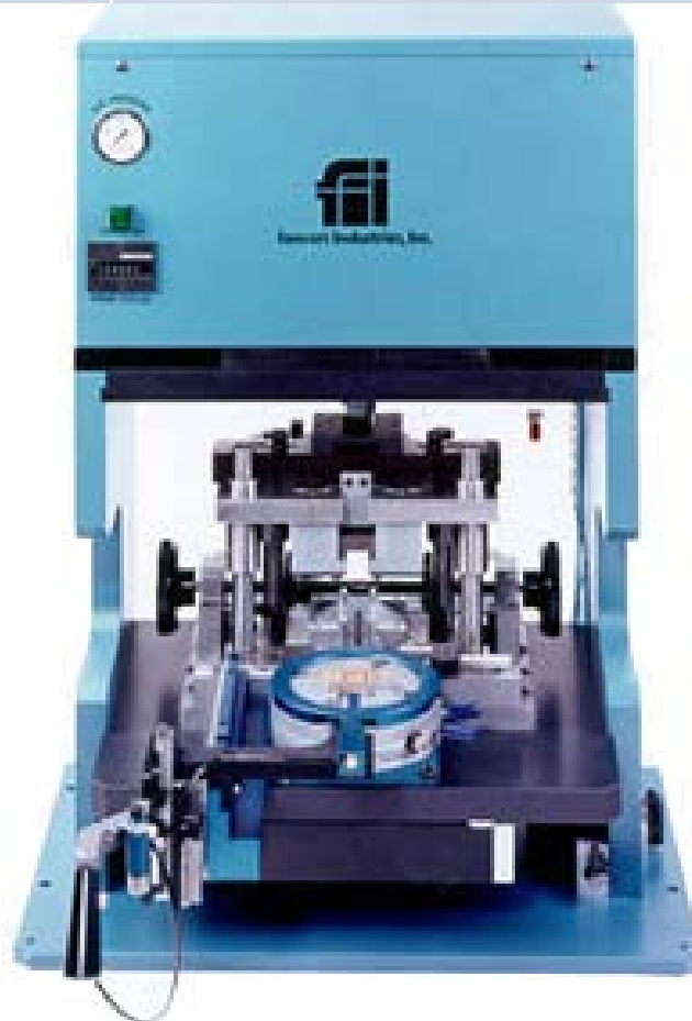
Part is lifted from the centering stage with the vacuum arm by the operator.
