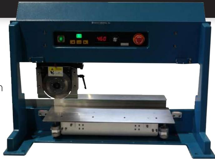
Separates .030"-.040" from score line without damage to components.
