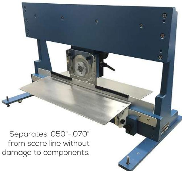
Separates .050"-.070" from score line without damage to components.
